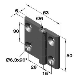
Art.no.: 4101 (perforated and countersunk) with stainless steel pin
