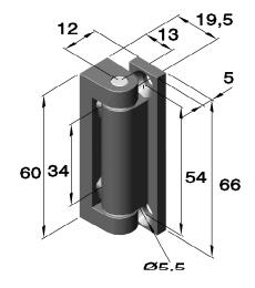
Art.no.: HS40 (drilled and countersunk)
