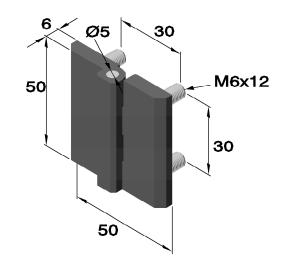
Art.no.: 4002 (with threaded pin) with pin in stainless steel
