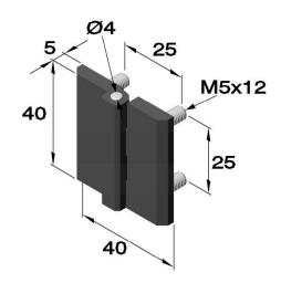
Art.no.: 4002 (with threaded pin) with pin in stainless steel
